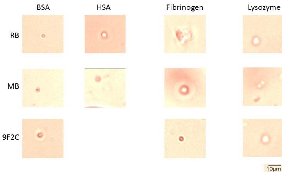
**Fig. 4.** Sample images of protein fabrications carried out with various photoactivators at a 20:1 concentration ratio. Exposure time was 10 seconds at a repetition rate of 10 Hz.
