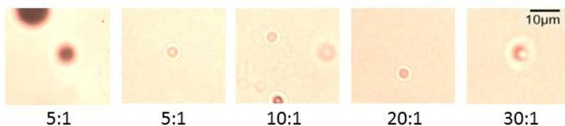
**Fig. 6.** Images of BSA/RB fabrication over a wide range of concentration ratios, with evidence of successful cross-linking and photodamage at 5:1. Some photodamage is also evident at 10:1.
